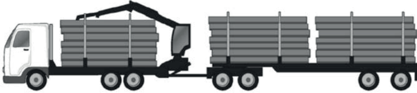
Figure 11. A typical self-loading logging truck and trailer combination under Swedish conditions is up to 24 metres long, and has a GVW of 60 tonnes (64 tonnes from June 2015). Copyright © 2016 Taylor & Francis.
