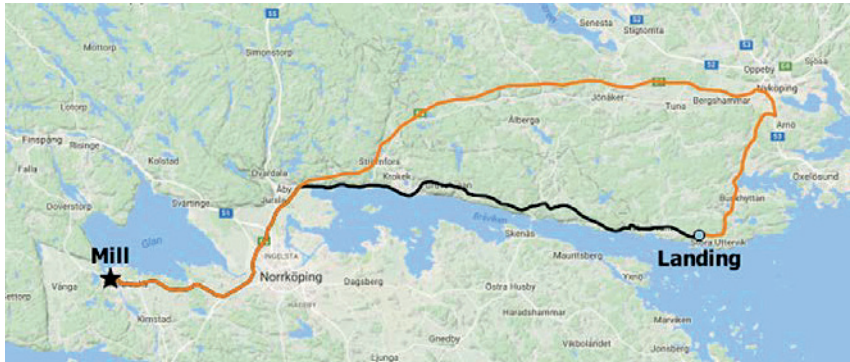
Figure 20. CRF chooses the minimum-cost route. In this example, the orange and the black route from landing to mill are similar in terms of resistance points, but they differ in length.
