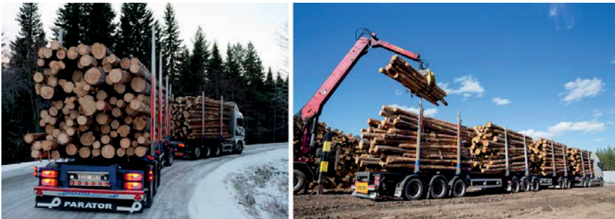
Figure 7. Two types of experimental trucks currently undergoing extensive trials and demonstration in Sweden. Left, a 74-tonne GVW self-loading truck with 9 axles and, right, the ETT 90-tonne GVW truck, with 11 axles distributed over the vehicle's total length of 30 metres. (Left photo, Niklas Fogdestam, right photo, Per Pettersson).
