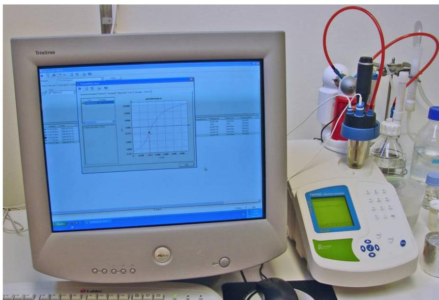
Figure 9. Laboratory setup of TIM960 Titration Manager coupled with PC and Titramaster 85 Titration Software. Sample was contained in an uncovered polyethylene vial; partial cover was provided by the electrode holder.
