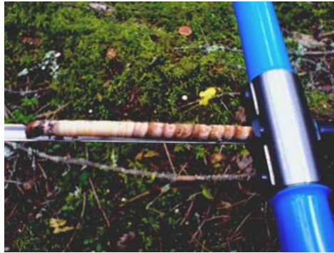
Figure 4. Collecting of wood sample using Presler increment borer.
