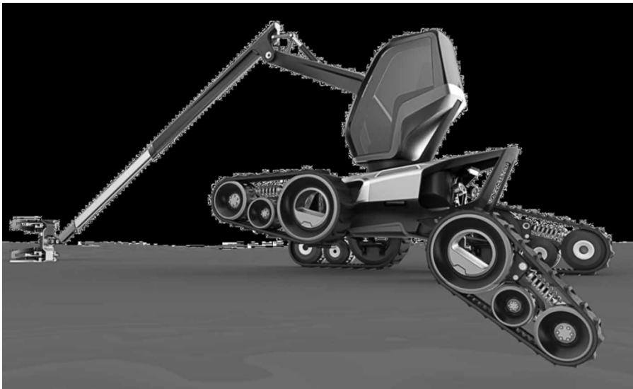
Figure 7: Illustration showing future possible developments with individually steerable wheels and a bogie concept that allows for adjustable contact area (Ross 2012).
