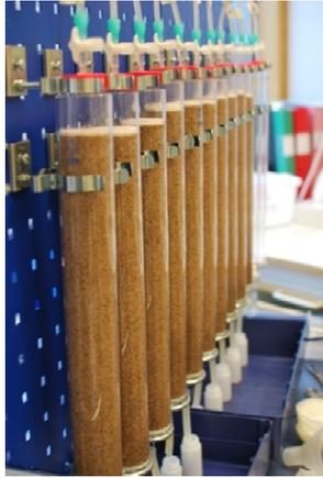
Figure 12. Equipment used for column studies of MCPA leaching.
