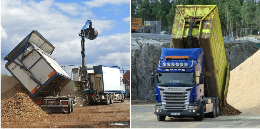
Figure 4. Fuel delivery with two different systems. Left: Truck using side-tipping of both truck and trailer. Right: Hook-lift truck emptying a bin with end-tipping.
