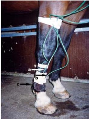
*Fig. 3.* Temperature probes adapted to a) subcutis, b) skin and c) fetlock joint of an equine forelimb.
