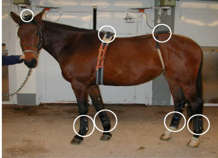
Fig. 5. Accelerometer devices adapted to the neck, withers, croup and legs.
