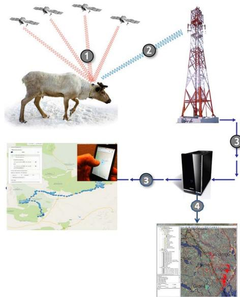
Figure 12 Reindeer are equipped with GPS collars that can provide hourly updates of movement in realtime. The system is supported through four inter-linked processes: 1. Reindeer are positioned with GPS and positions are stored in the collar. 2. Positions are sent as a text message via the cellular network. 3. Positions are displayed in real-time on web-based maps. 4. Positions are imported into RenGIS for analysis and visualization. Adopted from Sandström and Wedin (2010; Paper II).
