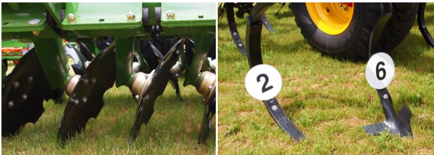
Figure 4 Discs (left picture) vs. tine and duckfoot (nr 2 and 6 in the right picture, respectively). Photos: Björn Ringselle
