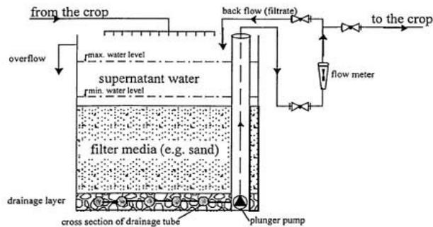
Figure 1. Schematic diagram of a slow sand filter used for horticultural purposes (Wohanka *cit.* Alsanius *et al.*, 2001).
