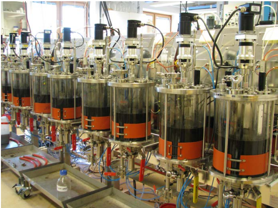
Figure 3. Laboratory-scale semi-continuous stirred tank reactor (CSTR).
