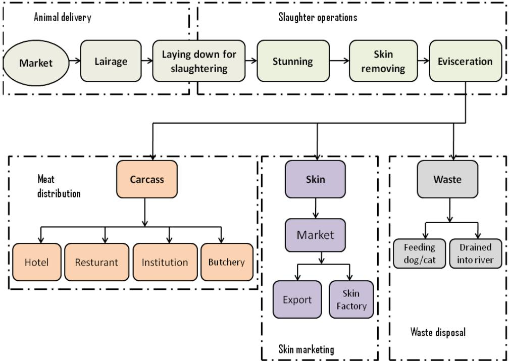
**Figure: 33. Operational structure of Ambo abattoir**
