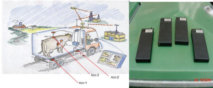
**Figure: 8. (a) Measurement sensors mounted on vehicle and animal to measure vibration levels and (b) loggers used to record vibration levels (diagram taken from Gebresenbet, 1997).**
