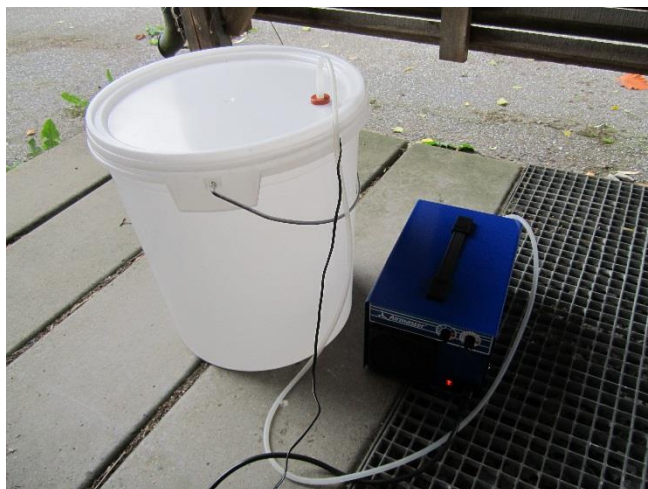
Figure 7. The sealed plastic jar connected with ozone generator.
