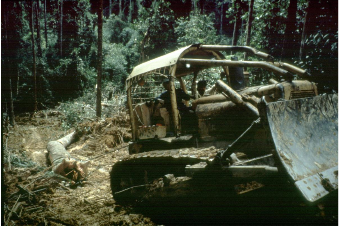
Crawler tractor extraction in selective logging in dipterocarp forest in Sabah, Malaysia (Photo Anders Malmer)
