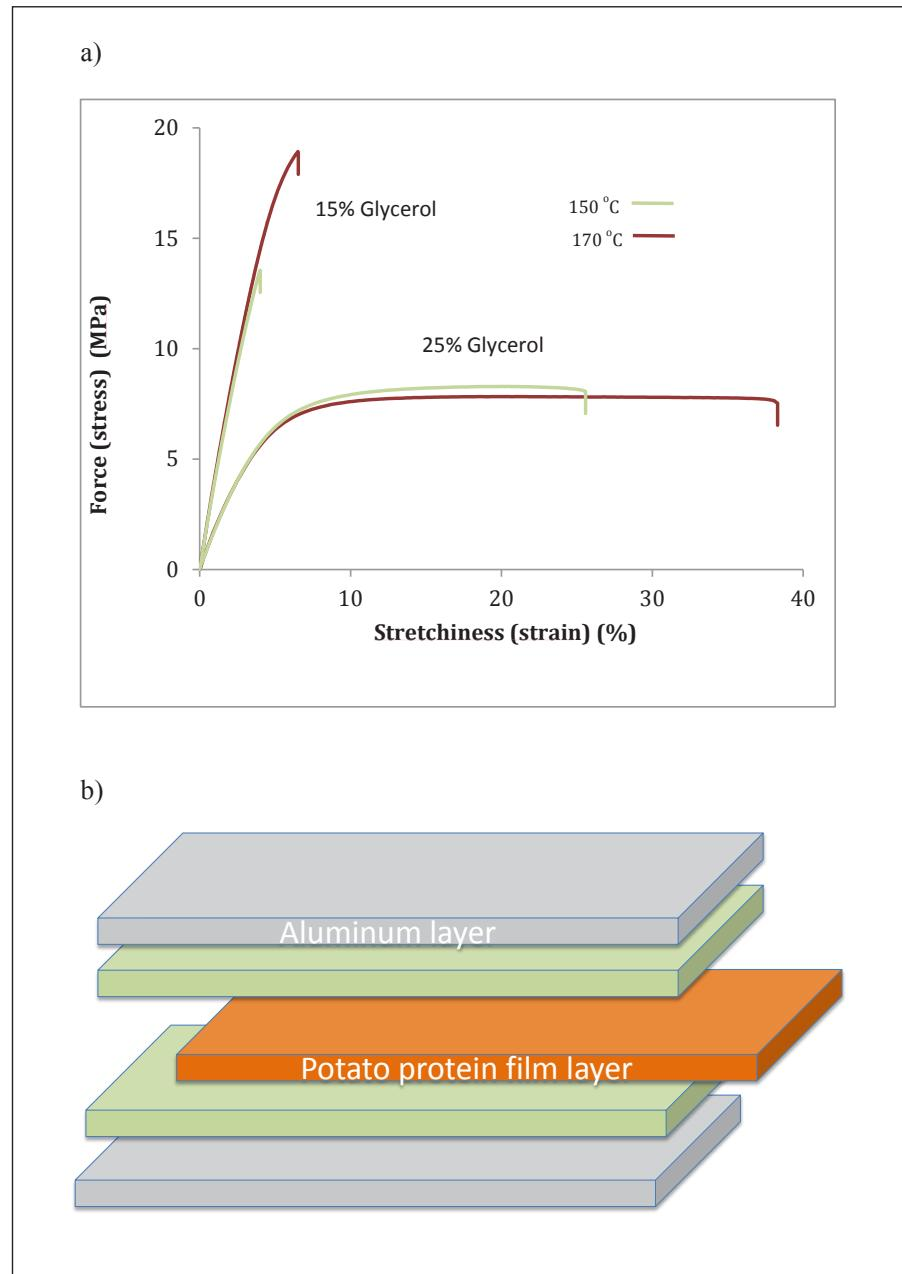
Figure 1 legend: a) Force (stress) and stretchiness (strain) for potato bioplastics formed with different amounts of plasticizer and at various processing temperatures, b) potato chip bag packaging example.
