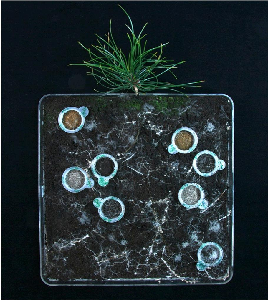
*Figure 20.* Laboratory microcosm for  $^{13}\text{C}$ -RNA stable isotope probing (SIP) studies.  $^{13}\text{CO}_2$  is fed to the central plant and patterns of carbon allocation to different fungi and bacteria colonising different substrates are followed by  $^{13}\text{C}$ -RNA SIP and 454 pyrosequencing.
