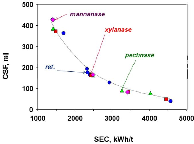
Figure 4. Freeness versus energy consumption for Wing-refining of batches of Impressafiner chips pre-treated with different enzymes for 60 minutes.
