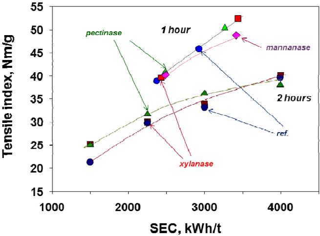
Figure 6. Tensile index versus energy consumption for Wing-refining of batches of Impressafiner chips pre-treated with different enzymes for either 60 or 120 minutes.
