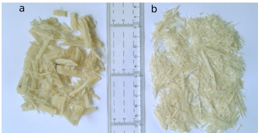
Figure 2. Visualization of the wood material of Norway spruce. a = Impressafiner chips, b = wood shavings.
