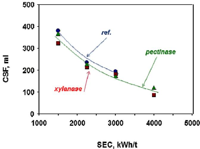
Figure 5. Freeness versus energy consumption for Wing-refining of batches of Impressafiner chips pre-treated with different enzymes for 120 minutes.
