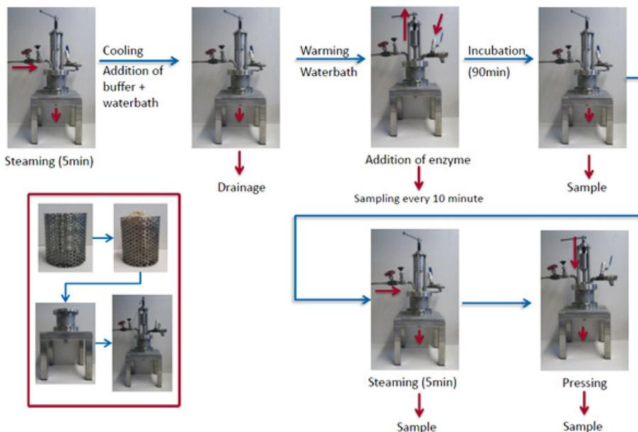
Figure 3. Visualization of wood chip pre-treatment in laboratory trials. The perforated container in the lower left corner was covered in a 200 mesh (74 $\mu$ m) net.
