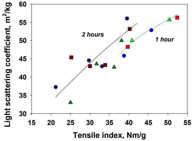
Figure 7. Light scattering coefficient versus tensile index for Wing-refining of batches of Impressafiner chips pre-treated with different enzymes for either 60 or 120 minutes. Circles – reference pulp; triangles – pectinase; squares – xylanase.
