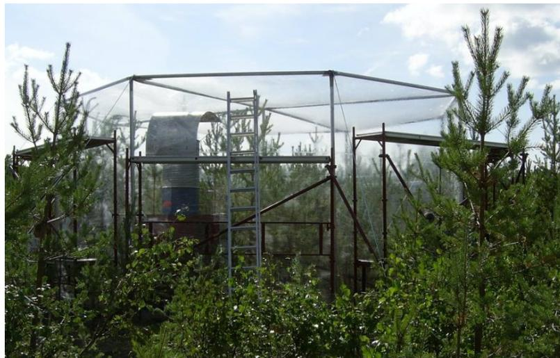
Figure 11. Photo of the 200  $\text{m}^3$  chamber that was used to label the canopy of young Scots pine trees with  $^{13}\text{CO}_2$ .
