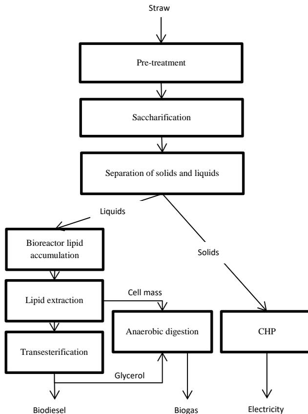
Figure 7. The biorefinery system considered in Papers IV and V.
