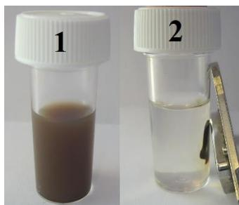
Figure 7. Core-shell  $\gamma$ -Fe<sub>2</sub>O<sub>3</sub>-SiO<sub>2</sub> NPs: 1) dispersed in ethanol ; 2) retracted by a magnet.
