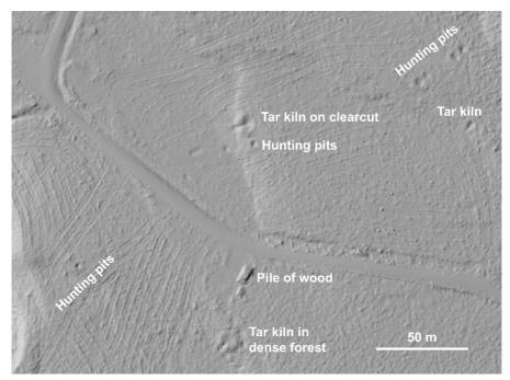
*Figure 6.* Section of the high-resolution DTM of the Krycklan study area, showing the cultural remains that were used for testing the parameters. The image shows the DTM as it was finally generated from a point-cloud that had been classified with relatively generous parameters, as shown by the wood pile by the road.
