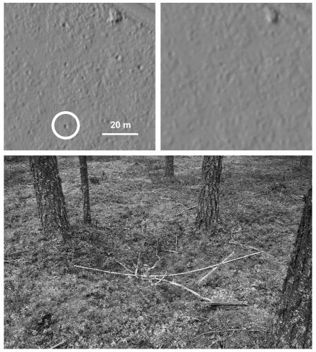
*Figure 21.* Stump pits were clearly visible in the HR DTM used in paper IV (upper left), but almost invisible in the DTM generated from the LR data set (upper right). The pit on the photo is the one encircled in the DTM. Since even such a shallow pit in closed forest is visible in the HR DTM, storage pits and roasting pits connected to Sami land use should also be detectable.
