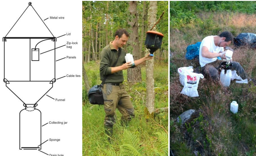
Figure 10. Schematic drawing of a flight-intercept trap (catch-release version), and the author servicing traps (drawing; M. Molander, photos: Bengt Lundberg, Björn Eriksson).
