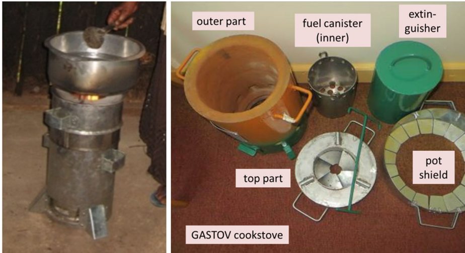
Fig. 1 Top-lit updraft (TLUD) gasifier cookstove used for combined cooking and char production. Left: the first version of the cookstove used in stages 1 and 2, which was made of steel sheets. Right: the second version of the cookstove (GASTOV) used in stage 3, which was slightly smaller and made of ceramics and steel
