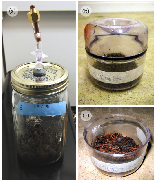
Figure 5. (a) shows jars used in Paper IV . The top end of the protrusion was fitted to evacuated flasks at gas sampling. (b) and (c) show incubation jars containing Norway spruce needles used in Paper II . (b) shows how the jar was stored between measurement occasions. In the bottom of the depression there is a small hole, enabling gas exchange whilst preventing too rapid water loss. Photos by the author.
