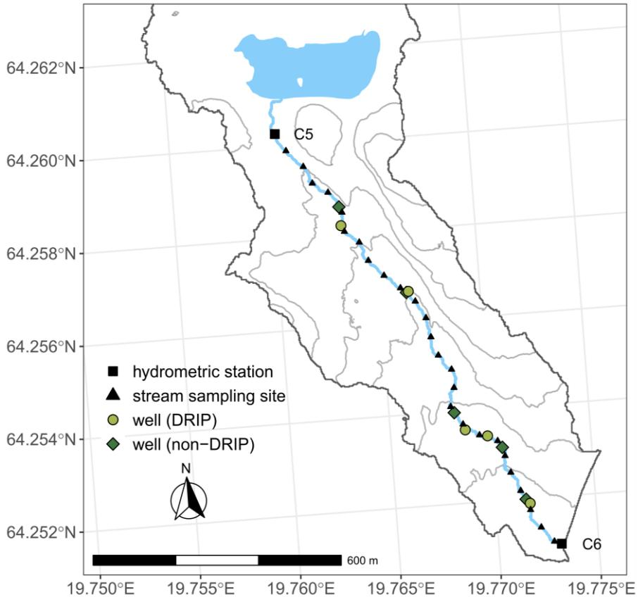
Figure 2 The C5-C6 stream reach. In black, squares indicate the hydrometric stations, and triangles show the stream sampling sites. DRIPs and non-DRIPs wells are indicated with light green circles and dark green diamonds, respectively. Figure adapted from paper IV.
