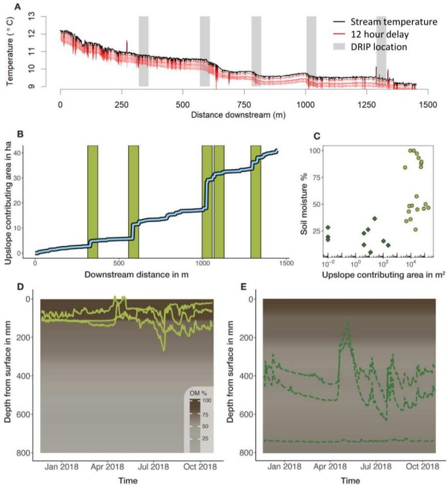
Figure 4 Overview of hydrological assessment of DRIPs. Panel A shows an example of a stream temperature profile from the DTS, with DRIPs indicated by grey bars. Panel B shows the change in UCA along the reach in blue and DRIPs in light green. In panel C soil moisture percentages are plotted against UCA, with DRIPs in light green circles and non-DRIPs in dark green diamonds. Panel D and E show groundwater levels of three
