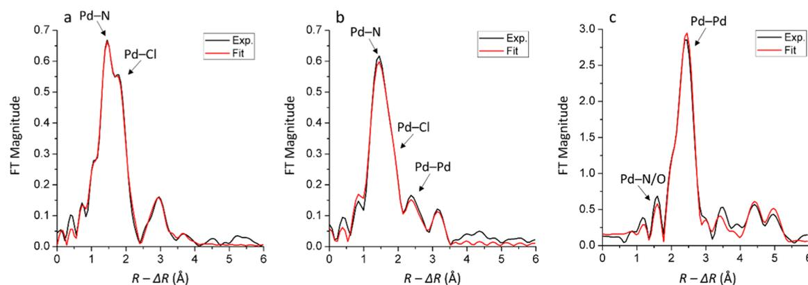
**Figure 3.** Fourier transformed  $k^3$ -weighted EXAFS spectra of (a) unused Pd(II)-AmP-MCF and the recycled catalysts (b) C1 and (c) C2. The spectra are not phase-corrected. The  $k$  ranges used to perform Fourier transform are 2–13, 2–10, and 2–12  $\text{\AA}^{-1}$ , respectively.
