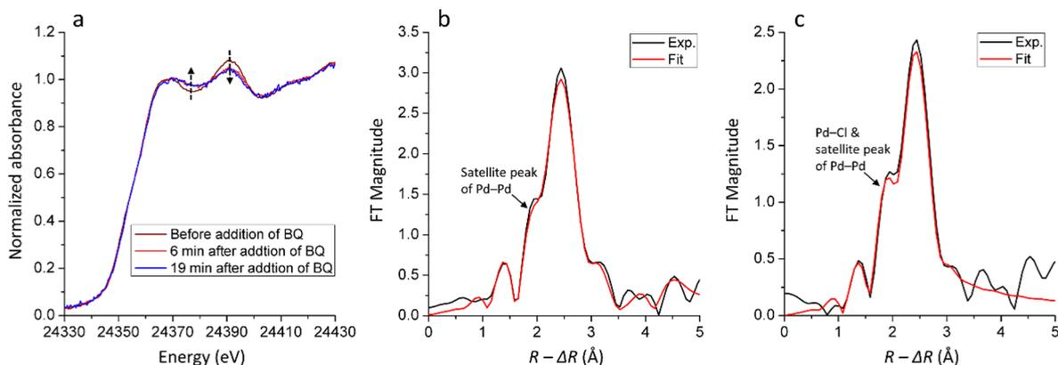
**Figure 6.** Representative *in situ* Pd K-edge (a) XANES spectra of the recycled catalyst from reaction with **S2**, (b) Fourier transformed  $k^3$ -weighted EXAFS spectra of the recycled catalyst from reaction with **S2** before addition of BQ and (c) after the addition of BQ. The spectra in (b) and (c) are not phase-corrected and are Fourier transformed in the same  $k$  range,  $2\text{--}10.5 \text{ \AA}^{-1}$ .
