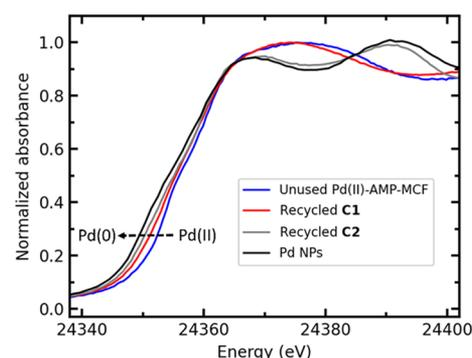
**Figure 1.** *Ex situ* Pd K-edge XANES spectra of unused Pd(II)-AmP-MCF, recycled C1 and C2, and the Pd NP reference. The Pd NP reference data is taken from ref 43.
