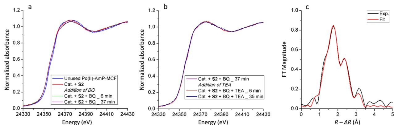
**Figure 8.** (a) Representative *in situ* Pd K-edge XANES spectra of Pd(II)-AmP-MCF after addition of S2 and BQ and (b) continued measurements of the XANES spectra from Figure 6a after the addition of TEA. (c) Fourier transformed  $k^3$ -weighted EXAFS spectrum of Pd(II)-AmP-MCF after the addition of BQ and TEA. The spectrum in Figure 6c is not phase-corrected and is Fourier transformed in the  $k$  range of 2–10  $\text{\AA}^{-1}$ .
