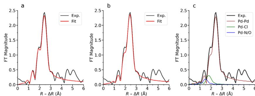
**Figure 7.** Fourier transformed  $k^3$ -weighted EXAFS spectra of the recycled catalyst from reaction with **S2** after the addition of BQ (a) with and (b) without introducing Pd-Cl single scattering and (c) single-scattering components used in the fitting. The spectra are not phase-corrected and are Fourier transformed in the same  $k$  range,  $2\text{--}10.5 \text{ \AA}^{-1}$ .
