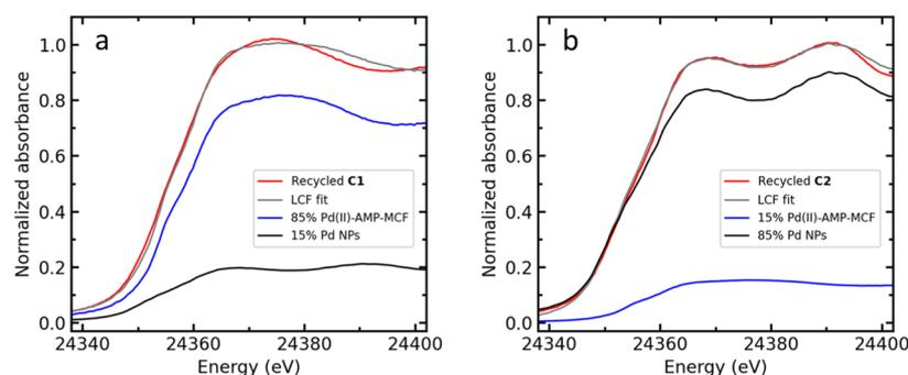
**Figure 2.** Linear combination fit of Pd K-edge XANES spectra of recycled (a) C1 and (b) C2. The XANES spectra of the Pd NPs and unused Pd(II)-AMP-MCF were used as the references for the metallic Pd component and the Pd(II) complex, respectively. All of the spectra used for the LCF are normalized and calibrated. Different weights of the references are iterated to find the best fit, while the sum of weights is always fixed at 1 and the  $E_0$  is not iterated in the fitting.<sup>12,44</sup>
