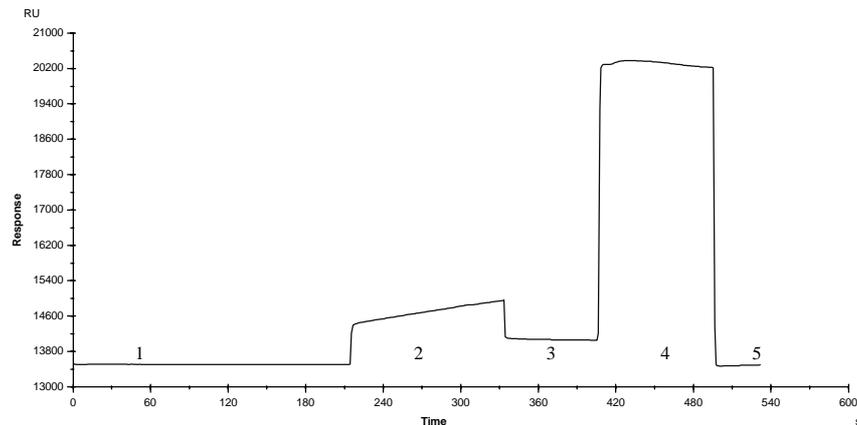
Figure 3. A sensorgram illustrating the interaction between free antibody in the sample and antigen immobilised to the surface. 1) baseline equilibrium (continuous buffer); 2) association of antibody to the sensor surface during injection; 3) response after injection of sample; 4) regeneration of the sensor surface; 5) baseline stabilisation.
