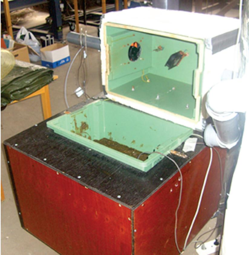
Figure 7. Climate controlled dynamic flux chamber where different air and manure temperatures were simulated for the experiments in Paper IV.
