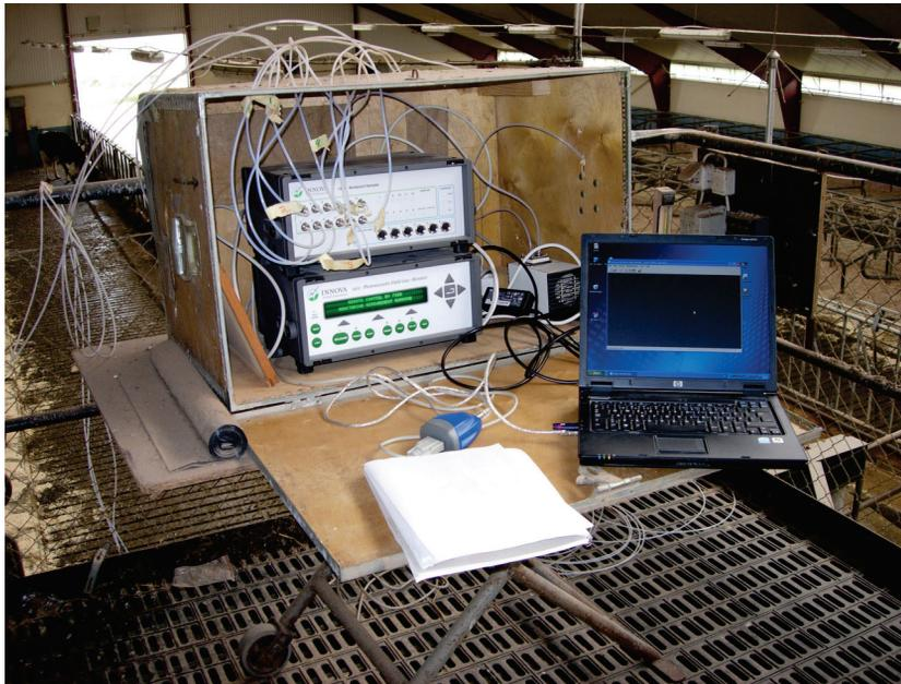
Figure 8. Photo-acoustic analyser coupled with a multiplexer during field measurements.
