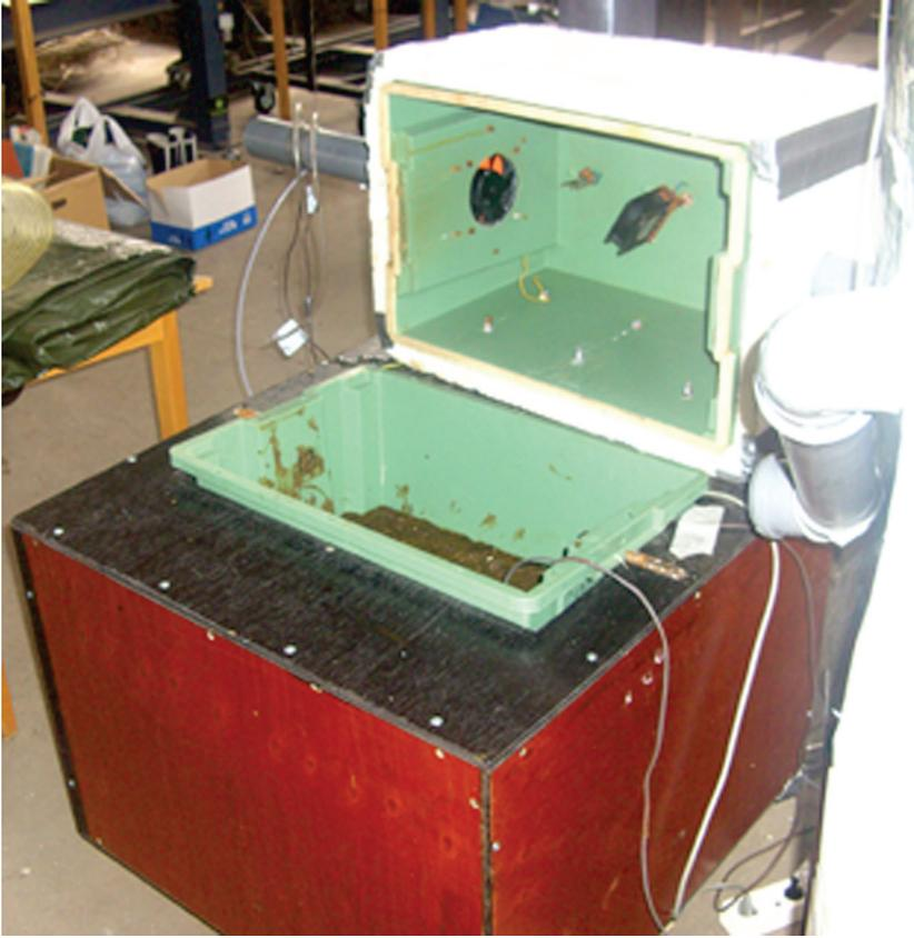
Figure 7. Climate controlled dynamic flux chamber where different air and manure temperatures were simulated for the experiments in Paper IV.
