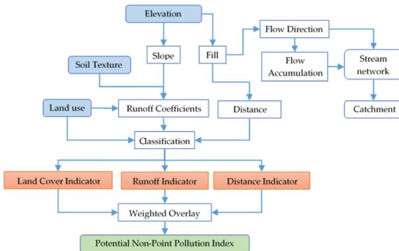
Figure 4. Workflow involved in calculation of Potential Non-point Pollution Index (PNPI).
