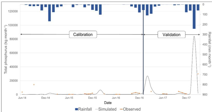
Figure 17. Comparison of observed and SWAT-simulated monthly total phosphorus and rainfall (2014-2016 calibration and 2017-2018 validation) in the Rocha River catchment.
