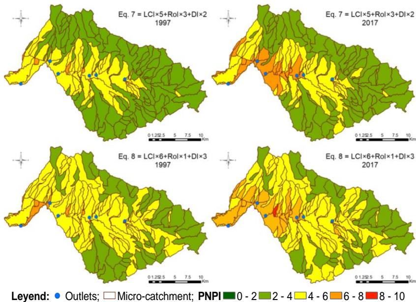
Figure 14. Spatial distribution of Potential Non-point Pollution Index (PNPI) classes at micro-catchment level in the Rocha River catchment in 1997 and 2017, calculated based on Equations (7) and (8).
