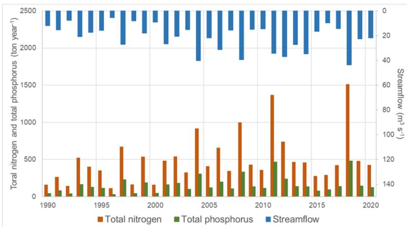
Figure 18. Simulated mean annual streamflow ( $m^3 s^{-1}$ ) and total nitrogen and total phosphorus (ton year $^{-1}$ ) in the Rocha River catchment in the study period 1990- 2020.
