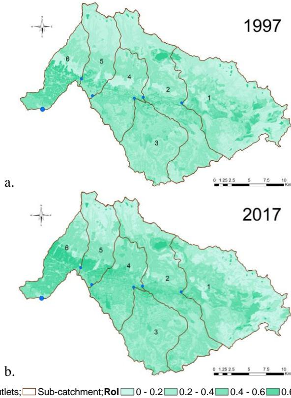
Figure 11. Runoff indicator (RoI) values for the Rocha River catchment in (a) 1997 and (b) 2017.
