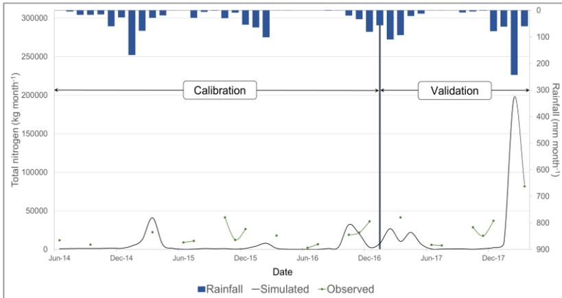
Figure 16. Comparison of observed and SWAT-simulated monthly total nitrogen and rainfall (2014-2016 calibration and 2017-2018 validation) in the Rocha River catchment.
