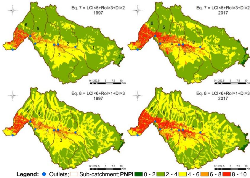
Figure 13. Spatial distribution of Potential Non-point Pollution Index (PNPI) classes in the Rocha River catchment in 1997 and 2017, calculated based on Equations (7) and (8).
