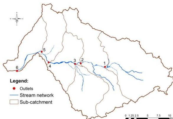
Figure 3. Sub-catchments of the Rocha River catchment and sub-catchment outlets where the six measuring stations were located.
