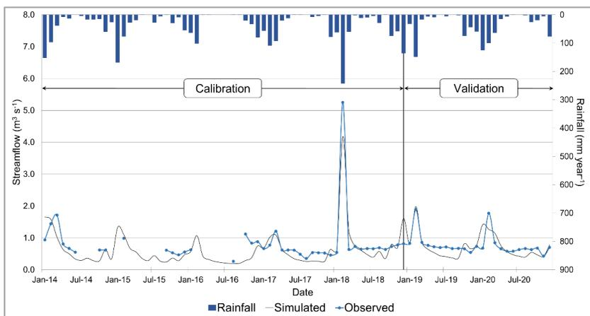
Figure 15. Comparison of observed and SWAT-simulated monthly streamflow and rainfall (2014-2018 calibration, 2019-2020 validation) in the Rocha River catchment.
