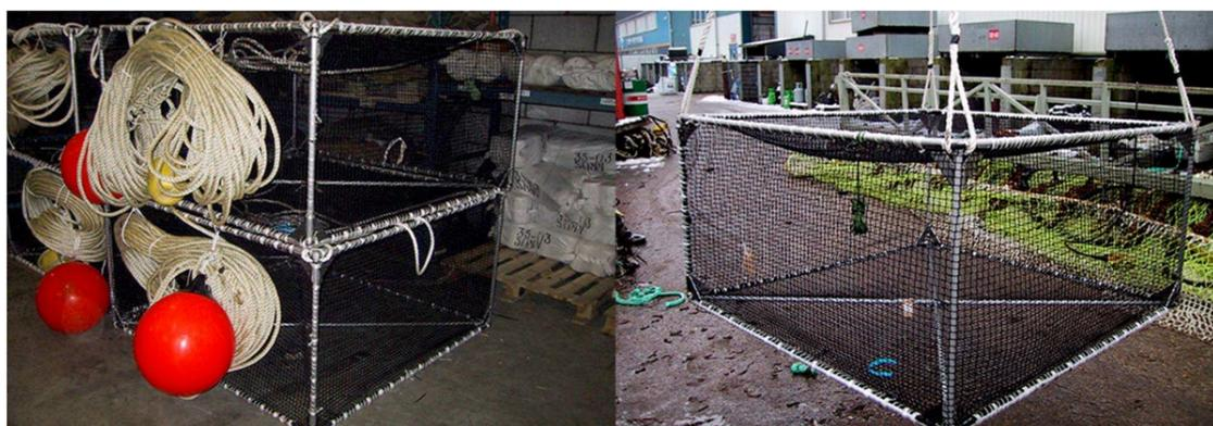
Figure 9.5. *In situ* sea cages for monitoring discarded catches out at sea on the seabed (Credit: Wageningen marine research, The Netherlands).
