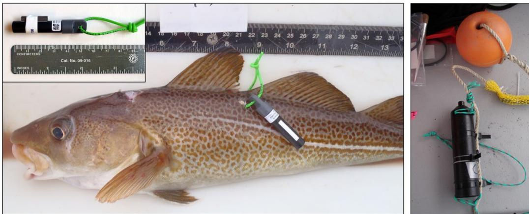
Figure 10.3. Top left: An acoustic transmitter externally attached to an Atlantic cod (*Gadus morhua*). Top right: The transmitter's signal is detected by an acoustic receiver. Bottom: Map depicting locations of acoustic receivers to passively monitor study area for tagged individual (reproduced from Capizzano *et al.* 2016).
