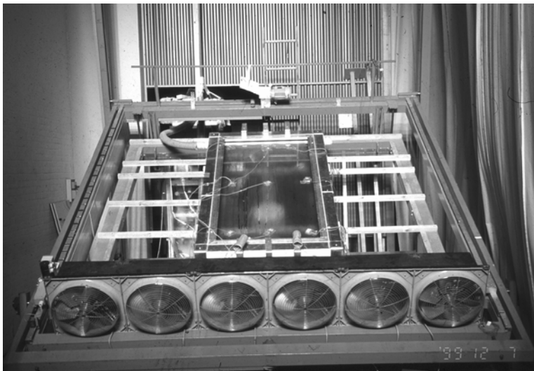
Fig.6. Laboratory experiment with the solar desalination module at the Department of Building and Energy, Technical University of Denmark.
