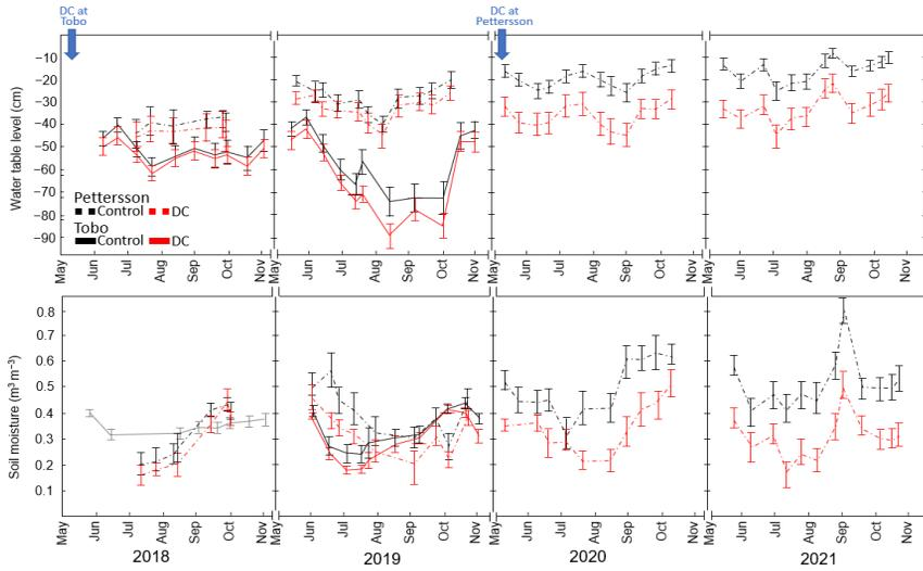
Figure 6. Time series of water table level (WTL) and soil moisture (SM) monitored at the measurement plots during flux measurements at the Pettersson (**Paper II**) and Tobo sites (**Paper II**). Data are averaged for each sampling event and grouped by experimental area (control versus DC) and year (2018–2021 for the Pettersson site and 2018–2019 for the Tobo site). The variable means for each sampling event  $\pm$  standard error (SE) are presented for both control and DC areas, respectively.
