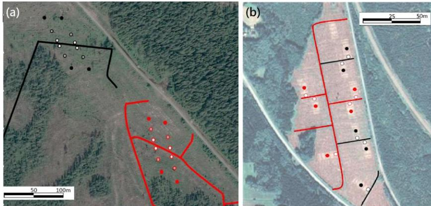
Figure 3. Map of ditch network at the (a) Pettersson and (b) Tobo field sites. Cleaned and uncleaned ditches are marked in red and black, respectively. The locations for manual chamber measurements are marked in red for the cleaned area and black for the uncleaned area (**Papers I and II**).
