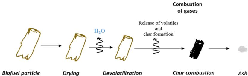
Figure 1. Simplified combustion stages of a solid biofuel particle.
