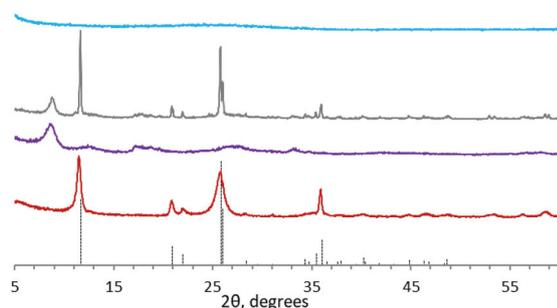
Fig. 2 Powder XRD patterns of the synthesised TiP products:  $\alpha$ TiP – sample 4, LTP-H – sample 3, TiP1-H – sample 1 and  $\alpha$ -TiP – sample 2 (adapted from ref. 35). The dotted line represents the referenced pattern of  $\alpha$ -TiP (ref. 4).
