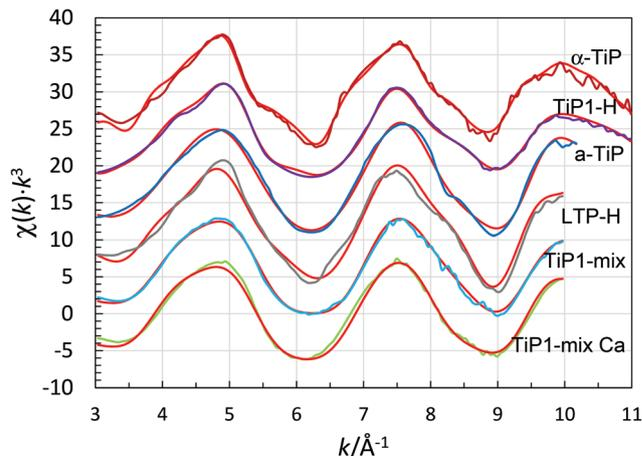
**Fig. 5** Fit of phosphorus K edge EXAFS data of titanium(IV) phosphates, experimental – coloured lines, models with structure parameters from Table 4 – red lines, sample 2 –  $\alpha$ -TiP (offset: 30), sample 1 – TiP1-H (offset: 24), sample 4 – aTiP (offset: 18), sample 3 – LTP-H (offset: 12), sample 9 – TiP1-mix (offset: 6), and sample 10 – TiP1-mixCa (no offset).
