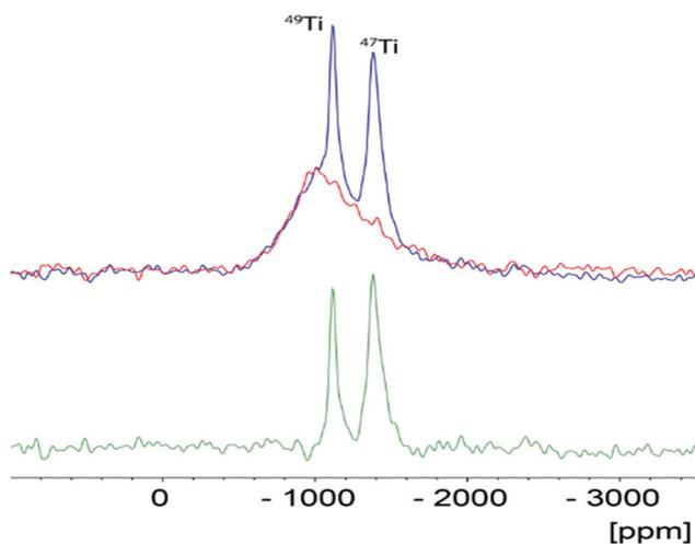
**Fig. 9** Static titanium NMR spectra of  $\text{TiP1-H}$  (red) and LTP-H (blue), scaled to the same height, and their difference (green). The resonances from both titanium isotopes,  $^{49}\text{Ti}$  and  $^{47}\text{Ti}$ , are clearly resolved in the difference spectrum.
