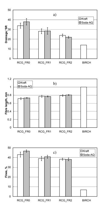
*Figure 4.* a) drainage, b) fibre length, and c) fines content of RCG pulp produced at different degrees of fractionation with the kraft and soda-AQ processes. RCG\_FR0 indicates no fractionation, RCG\_FR1 fractionation with one stage separation, and RCG\_FR2 fractionation with two-stage separation. The error bars indicate  $\pm$  the standard deviation of the measurements.
