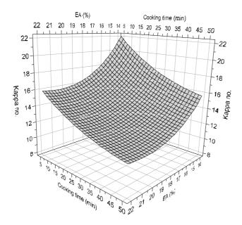
*Figure 7b.* Kappa number as a function of alkali charge and cooking time for the soda-AQ process. Two-stage fractionated RCG.
