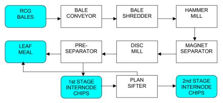
Figure 3. Schematic overview of the dry fractionation process developed by UMS A/S.
