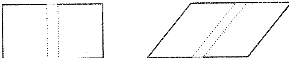
Fig. 1. Section of a soil element with a channel embedded. Left: original shape. Right: shape after shear strain at constant volume.
