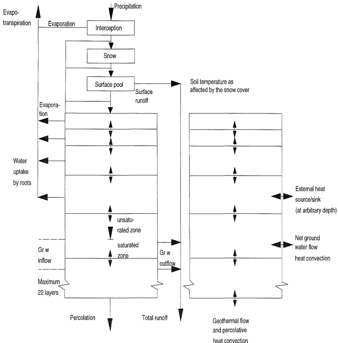
Mass balance (left) and heat balance (right) of the SOIL model.
