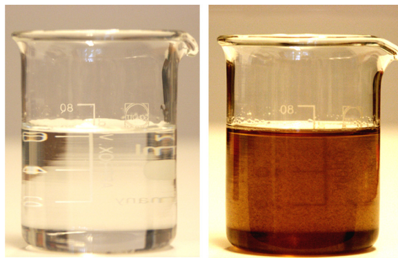
Fig. 3. Log yard run-off from an open sprinkling system (to the right) and tap water for comparison.
