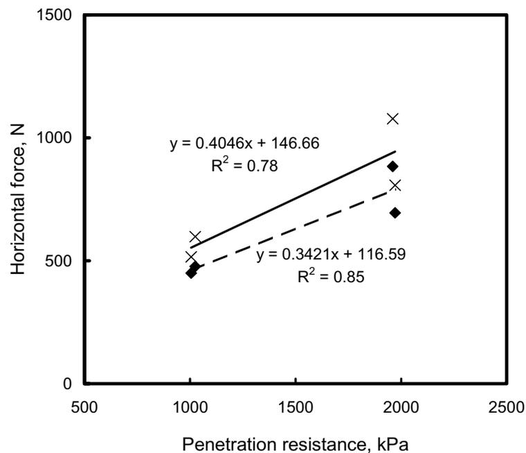
Fig. 23. Correlation between soil strength measured with a penetrometer and horizontal forces for the tines: ◆, double disc tine (DD); ×, the small tubulator tine with sharp tip (TSSh) at four soil conditions at 5 cm depth.
