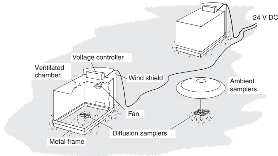
*Fig. 9.* Experimental apparatus for measuring ammonia emissions after land spreading of manure (Rodhe & Karlsson, 2002).
