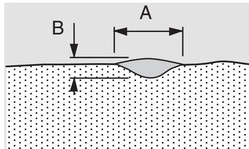
Fig. 8. Measurement of slurry placement in the soil after spreading; A, width; B, depth.
