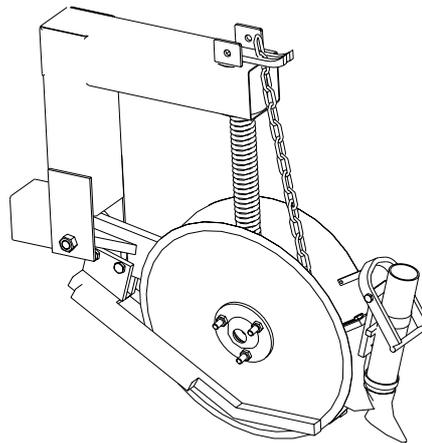
*Fig. 5.* Double disc tine (DD) consisting of two angled disc coultters with diameter of 0.40 m followed by a slurry outlet.
