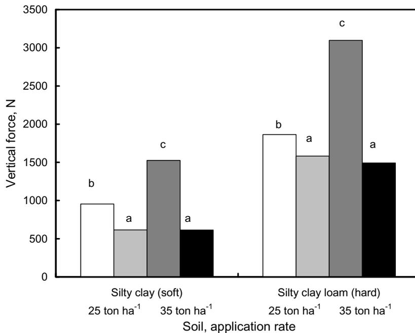
Fig. 22. Vertical forces (Least Significant Means), [N] for tines used at two different soil conditions; for 25 t ha<sup>-1</sup>: □, double disc (DD) at 5 cm depth; ▒, small tubulator with sharp tip (TSSh) at 5 cm depth; and for 35 t ha<sup>-1</sup>: ■, double disc (DD) at 8 cm depth; ■, medium tubulator with sharp tip (TMSh) at 5 cm depth. Averages with different letters (a-d) within each group are significantly different (probability  $P < 0.05$ ).
