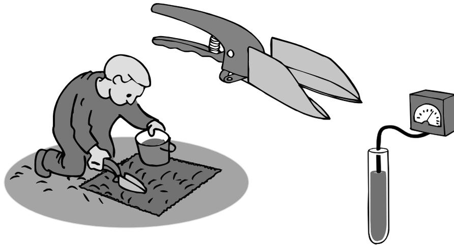
Fig. 7. Measuring contamination of the stubble by sampling and EC-measurements.
