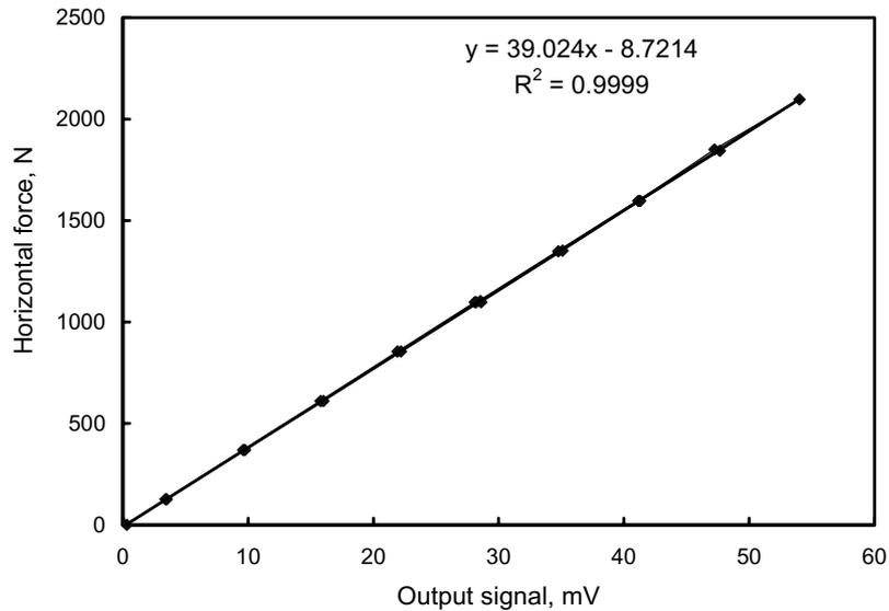
Fig. 13. Calibration curve of the octagonal ring sensor with a regression line for output signal and horizontal force ( $F_x$ ) applied.
