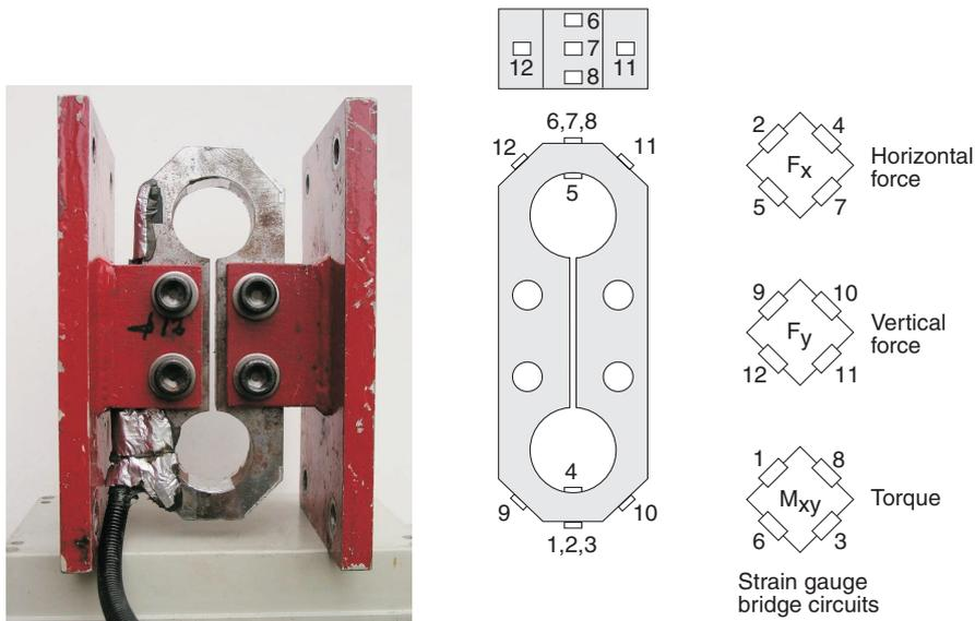
Fig. 12. The octagonal ring sensor with the placement of the strain gauges on the steel body and connection in full bridges.
