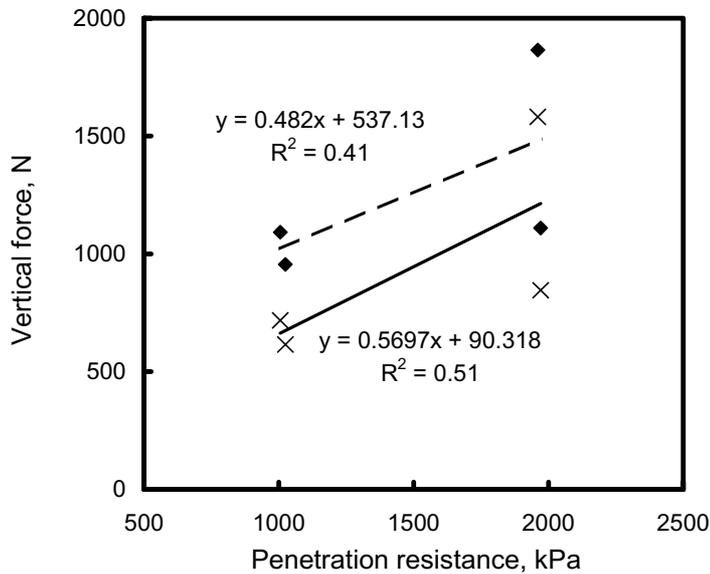
Fig. 24. Correlation between soil strength measured with a penetrometer and vertical forces for the tines: ◆, double disc tine (DD); ×, the smallest tubulator tine with sharp tip (TSSh) at four soil conditions at 5 cm depth.
