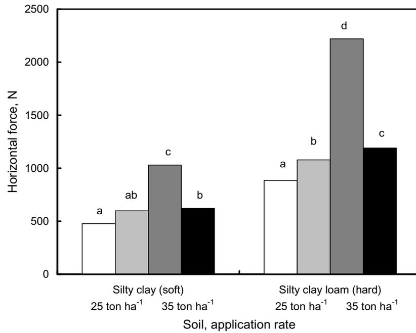
Fig. 21. Horizontal forces (Least Significant Means), [N] for tines used at two different soil conditions; for 25 t ha<sup>-1</sup>: □, double disc (DD) at 5 cm depth; ▒, small tubulator with sharp tip (TSSh) at 5 cm depth; and for 35 t ha<sup>-1</sup>: ▓, double disc (DD) at 8 cm depth; ■, medium tubulator with sharp tip (TMSH) at 5 cm depth. Averages with different letters (a-d) within each group are significantly different (probability P < 0.05).
