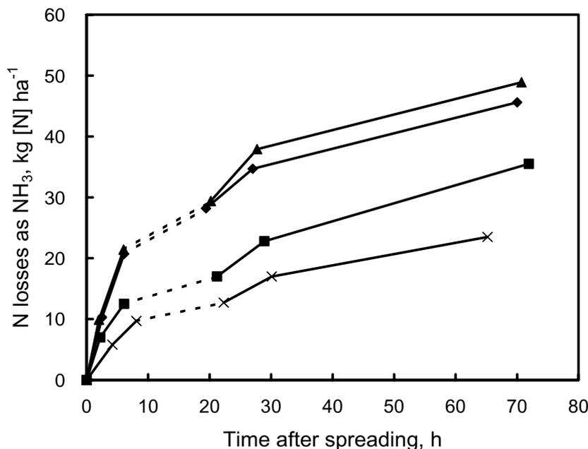
Fig. 17. Year 2, Paper III. Cumulative nitrogen losses as ammonia after spreading of cattle slurry on ley using the three different methods; periods of ammonia measurement are marked with solid lines; during periods marked with dotted lines, the ammonia emissions were interpolated and corrected for the prevailing weather conditions: ◆, band spreading; ■, pressurised injection; ▲, shallow injection 1; ×, shallow injection 2 (Paper III).
