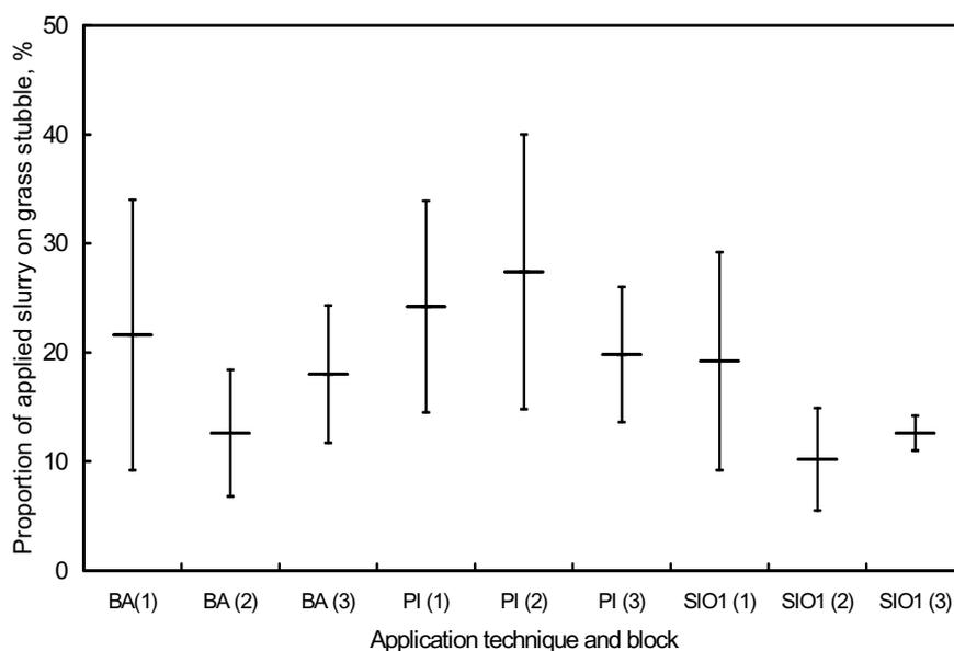
Fig. 14. Average proportion of slurry contamination of stubble after application of slurry on ley with three different techniques (three replicates, 1 to 3): band application (BA), pressurised injection (PI), and shallow injection 1 (SIO1) with open slots, V-shaped disc tines. Standard deviation represented by vertical lines (Year 1, Paper II).
