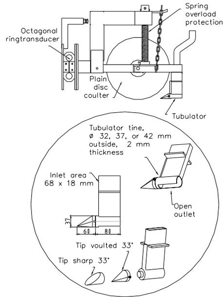
*Fig. 4.* The tubulator with a plain disc coultter followed by a tine consisting of different combinations of three dimensions and two types of tips (6 designs); in addition, the plain disc coultter (PD) was studied on its own.
