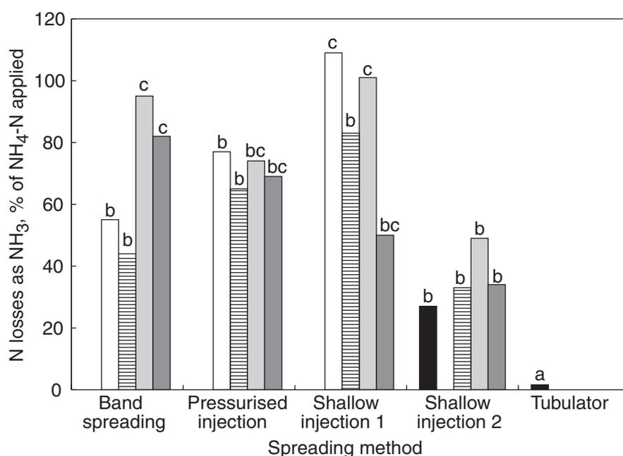
Fig. 16. Nitrogen losses as ammonia (% of applied NH<sub>4</sub>-N) after spreading of cattle slurry with five different techniques from five different experiments (Papers II-IV). □, year 1, Paper II; ▨, year 1, Paper III; ▤, year 2, Paper III; ▥, year 3, Paper III; ■, Paper IV. Means with different letters within each experiment are significantly different ( $P < 0.05$ ).
