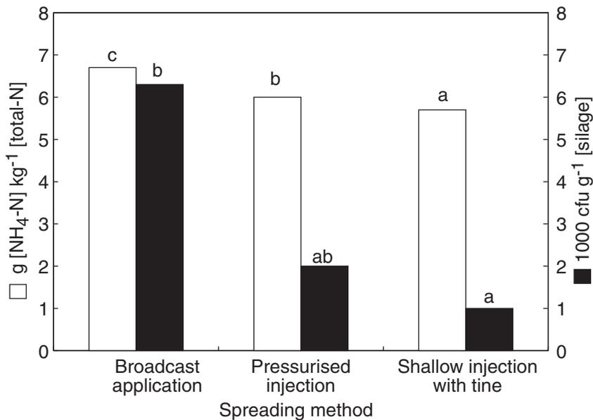
Fig. 19. Content of ammonia-N and colony forming units (CFU) of clostridia spores (1000 CFU g<sup>-1</sup>) in silage after 100 days of storage. Slurry applied with different application methods (Paper II); bars for each content category with different letters are significantly different ( $P < 0.05$ ).
