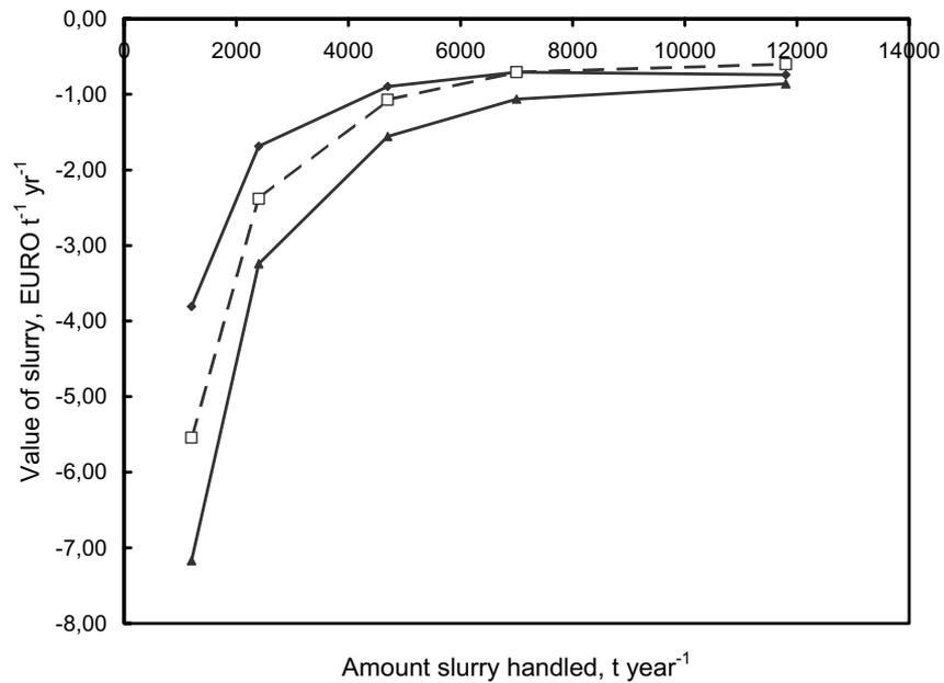
Fig. 20. Maximised net present value (€/year) per tonne of cattle slurry handled and spread with different methods; costs for storage are not included; load capacity of tanker 15 m<sup>3</sup>: ◆, broadcast spreading; ■, band spreading; ▲, shallow injection.
