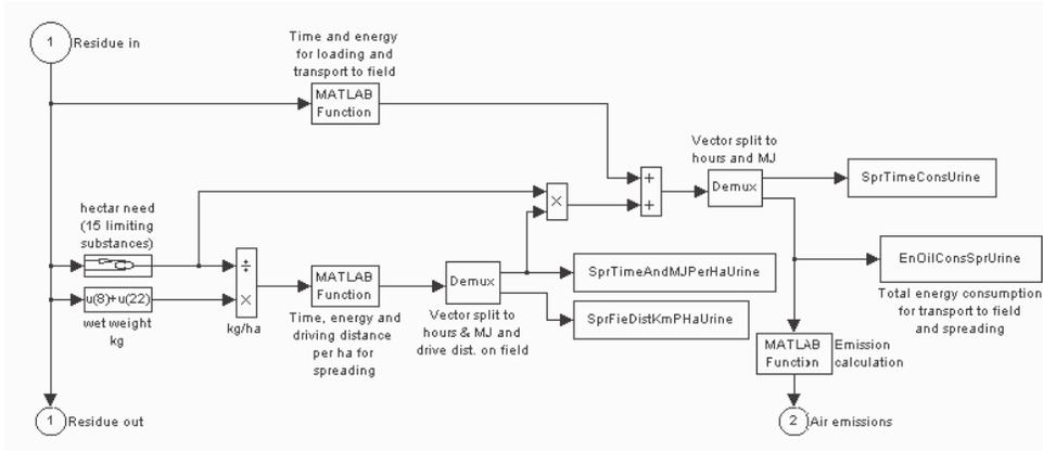
Figure 20. The liquid manure spreader sub-model.
