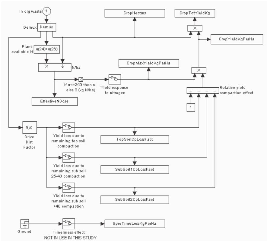
Figure 23. The grain production sub-model.
