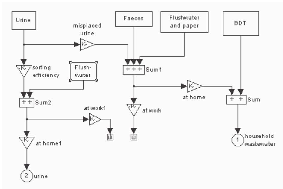
Figure 11. The household wastewater (with urine separation) initialisation block.
