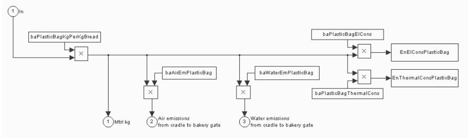
Figure 60. Plastic bag production sub-model.
