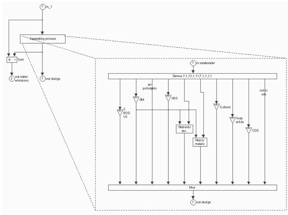
Figure 13. The sludge separation sub-model. Upper level at left, lower level at right.
