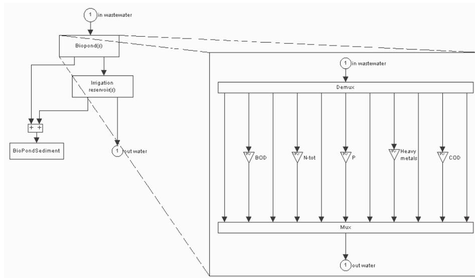
Figure 15. The biopond sub-model. Upper level at left, lower level at right.
