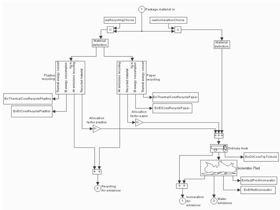
Figure 61. General structure of the packaging waste handling sub-model.
