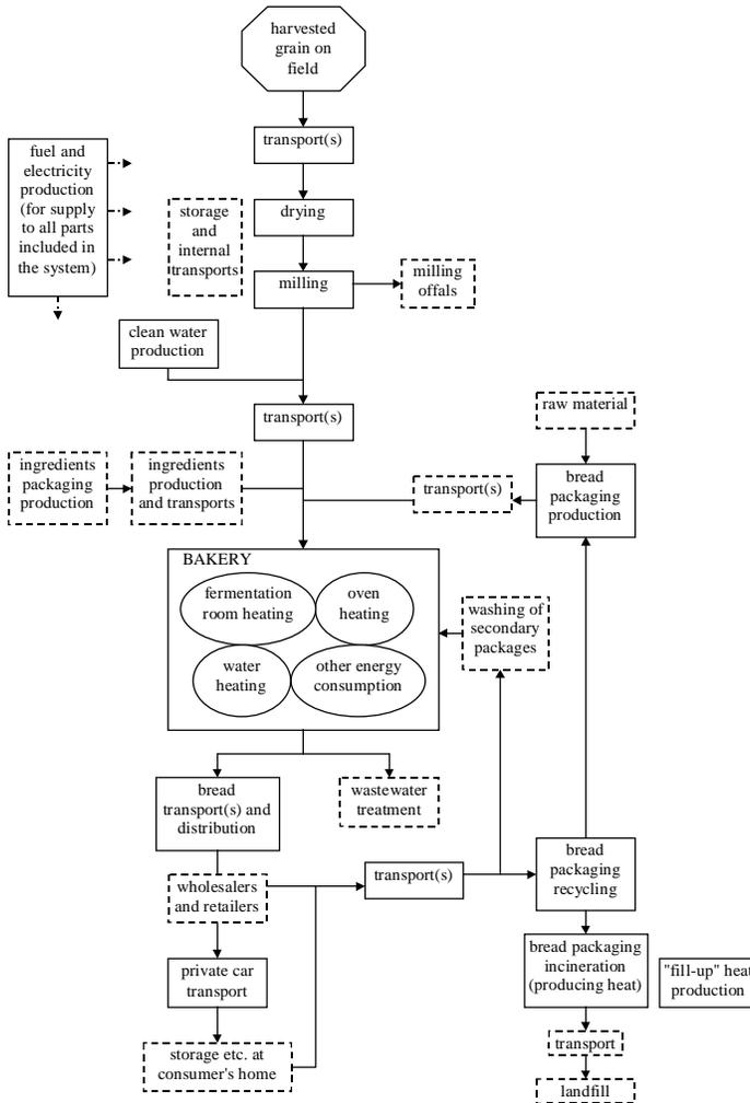
Figure 54. Flow chart of the bread production system. Dotted blocks not included in the study.
