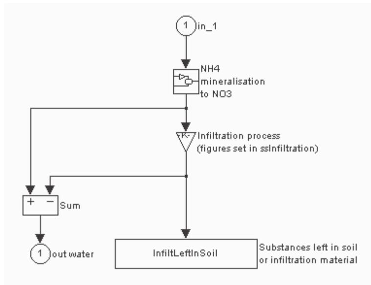
Figure 14. The infiltration sub-model.
