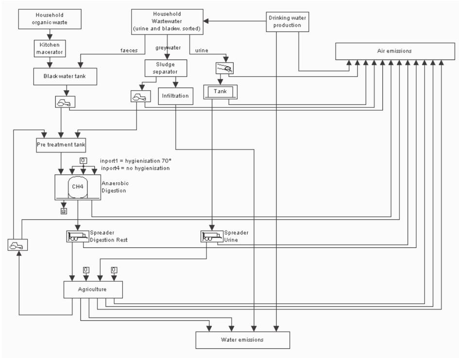
Figure 9. General structure of the organic waste management model. The anaerobic digestion with urine separation scenario.
