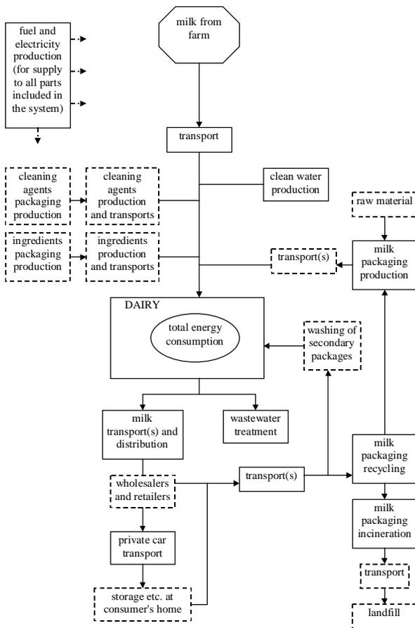
Figure 78. Flow chart of the milk production system. Dotted blocks not included in the study.
