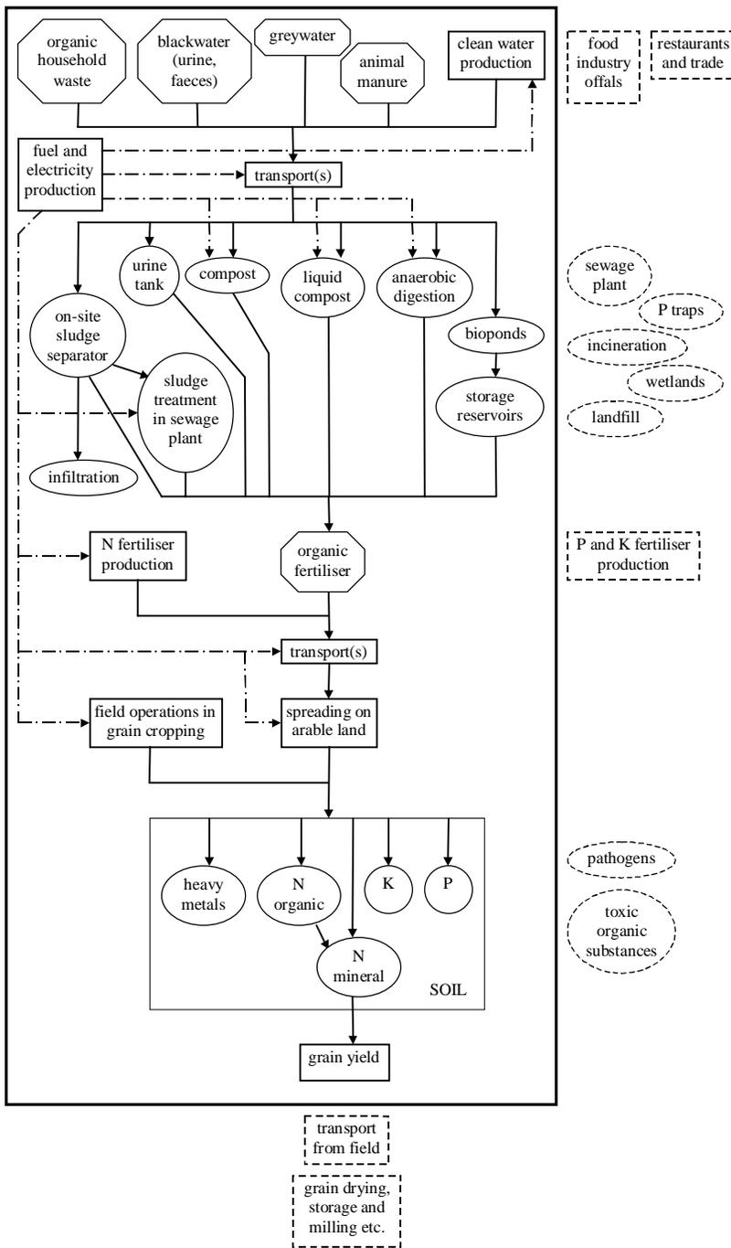
Figure 7. Parts included and system boundary in the organic waste management study.
