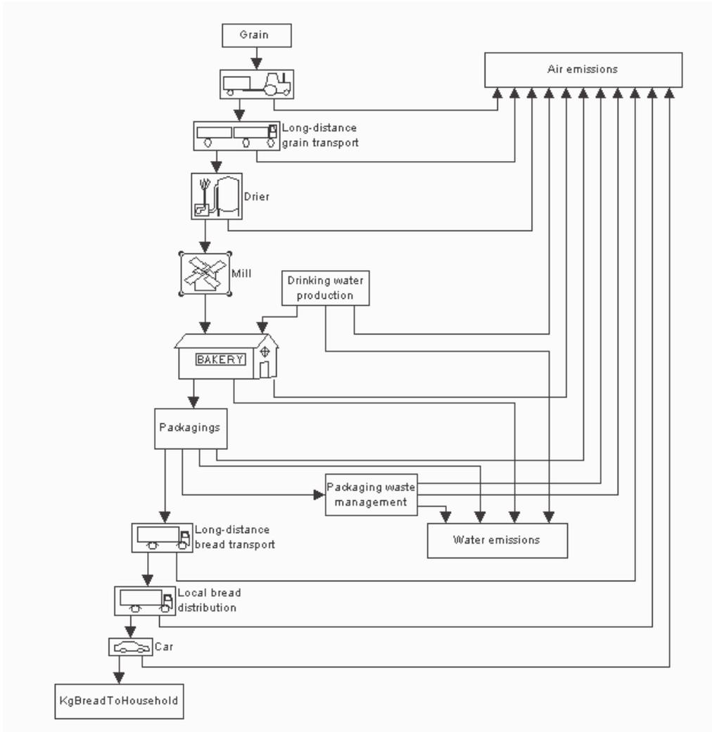
Figure 55. General structure of the bread production system model.
