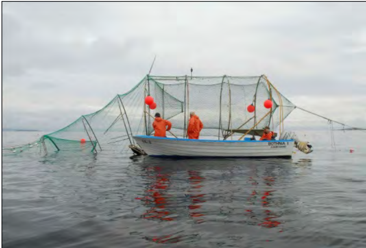
Fig. 4. Pontoon fish chamber lifted to the surface.
