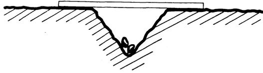
Fig. 2. The seeds have not been bedded down, but, despite this, they are protected against evaporation by the glass pane. The light has free access to the seeds.
