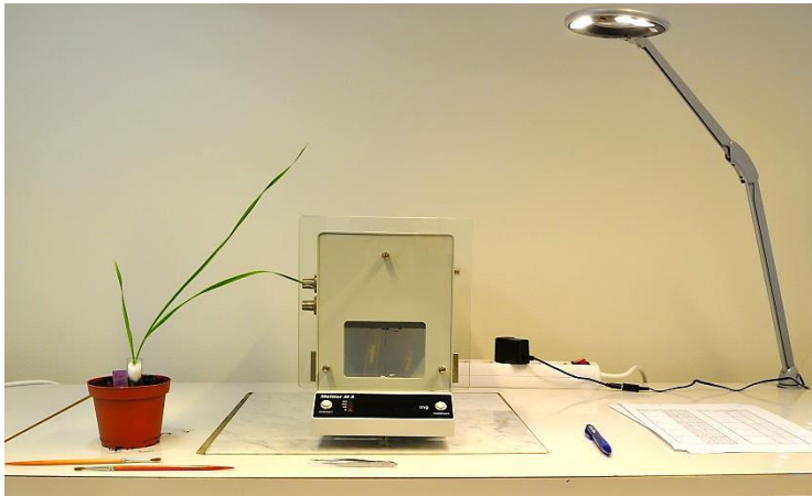
Figure 2. Wheat seedling infested with Rhopalosiphum padi nymphs 4 days prior to weighing on a microbalance to calculate aphid growth relative to that on a control plant.
