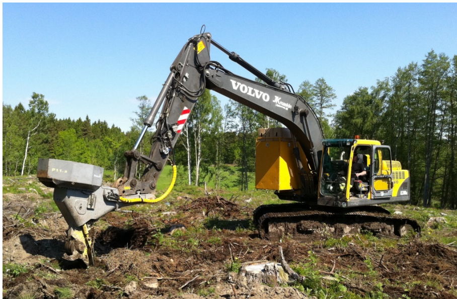
Figure 7. One of the four tree planting machines contracted by Södra Skog in 2013. All four machines consist of a medium-sized tracked excavator with a crane-mounted Bracke Planter planting device. This contractor purchased his device in 1994 and has been planting with it ever since (e.g. in the UK during the trials of Drake-Brockman, 1998), although completely refurbishing it once and upgrading to newer excavators over the years.
