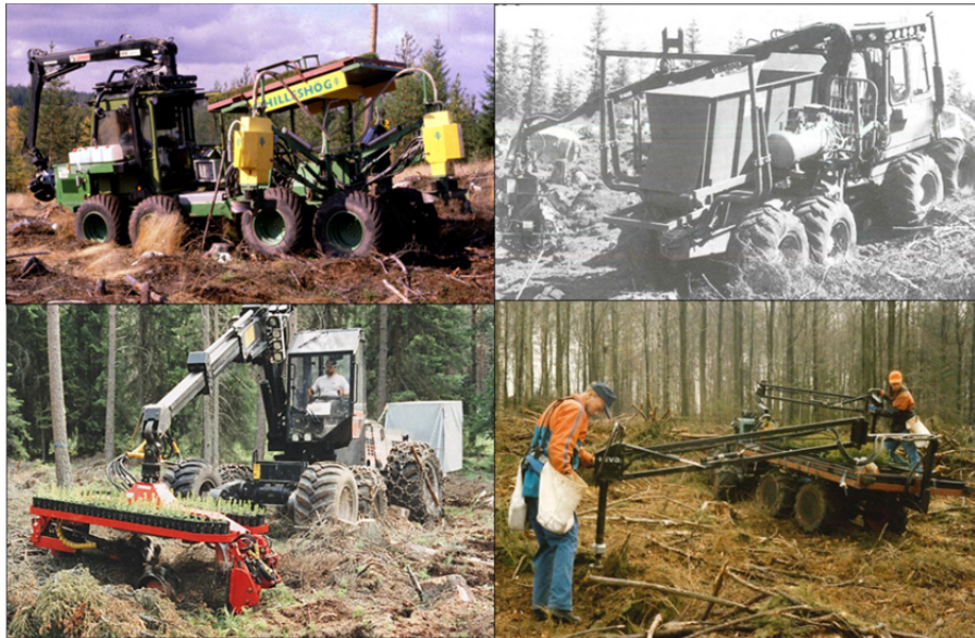
Figure 6. Intermittently advancing Nordic tree planting machines of the past: the forward-mounted, three-rowed Hiko/Hilleshög planting unit (top left); the crane-mounted, one-headed Doppingen planting device which planted using extra-added soil (top right); the crane-mounted, two-headed EcoPlanter planting device carried by a harvester (bottom left); the semi-mechanized Hevotrac planting machine with two manually operated planting drills (bottom right). Photos from SLU's Skogsbibliotekets bildarkiv, Adelsköld and Myhrman (1985), Staffan Mattson/Skogforsk, and Henrik von Hofsten/Skogforsk, respectively.
