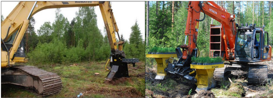
Figure 8. Crane-mounted planting devices currently manufactured and used in Finland, the one-headed Risutec (left) and two-headed M-Planter (right). Photos from Risutec Oy and Heidi Hallongren, respectively.
