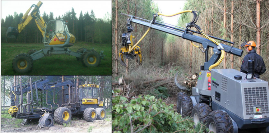
Figure 31. Upper left: the Menzi Muck A91 all-terrain excavator, an example of a wheeled excavator suitable for forest terrain (photo: Niklas Bodén). Lower left: Pentin Paja's modified forwarder that potentially might serve as the base machine for a continuously advancing planting machine (photo from Saarinen et al. , 2013). Right: the Forest Ebeaver, an example of a small, remote-controlled base machine that could serve as the prime mover for semi-autonomous planting-only machines in the future (photo from Key, 2012).
