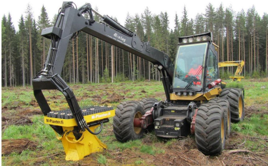
Figure 32. A six-wheeled Ecolog harvester with a one-headed M-Planter device and modified outer boom working as a tree planting machine in Finland (photo: Tiina Laine).
