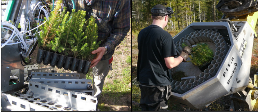
Figure 21. Left: tray-wise loading of a Hiko cultivation tray onto one of MagMat's eight frames (Photo: Rikard Wennberg). Right: seedling-wise loading of today's standard Bracke Planter carousel (note: the right-hand picture was not taken during the time studies).
