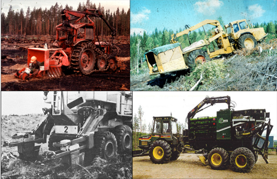
Figure 5. Continuously advancing Nordic tree planting machines of the past: the tractor-drawn YLÖ/Finn Forester planting unit with a one-row, continuously ploughing planting head (top left); the forwarder-mounted, two-rowed SHS V planting unit with intermittently ploughing planting heads (top right); the forwarder-mounted, two-rowed Serlachius planting unit with dibbles on glide bars (bottom left); the forwarder-mounted, two-rowed Silva Nova planting unit with dibbles on planting arms (bottom right). Top row photos from Skogsbibliotekets bildarkiv, SLU. Bottom row photos from Stjernberg (1985) and Åhlund (1995) respectively.
