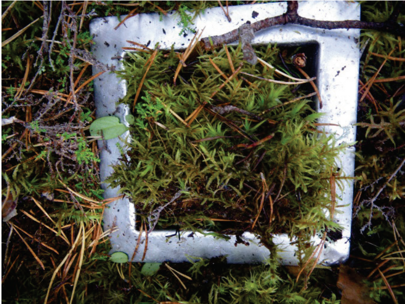
Figure 7. Soil corer used for extraction of litter layer in the pine forest ( paper II ). Photo: L.A. Widenfalk
