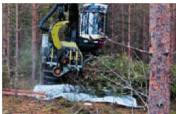
Figure 34. The “MAMA” head used in field trials for processing a bunch of trees on a blanket to collect the scraped-off biomass.
