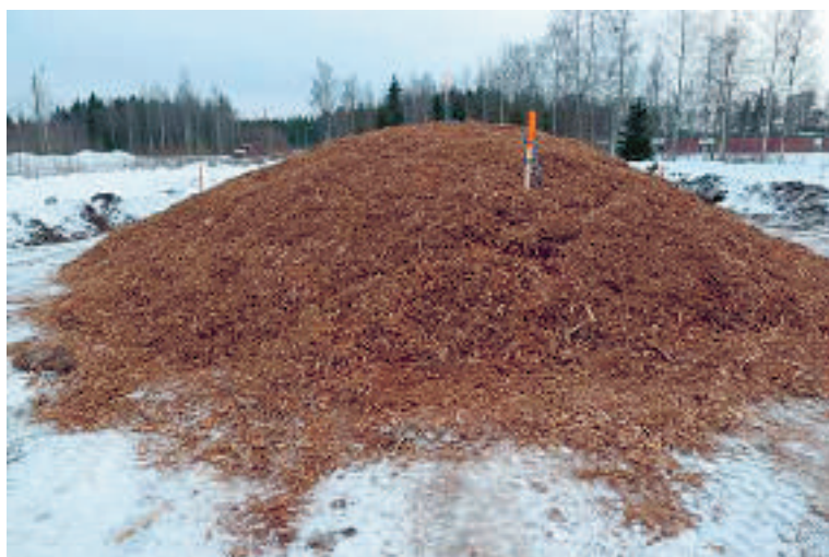
Figure 49. Pile of birch bark at UPM Pietarsaari mill. The sample taken for analysing suberin was taken immediately after the wet debarking. The pile in this photo was constructed for the storage experiment in which changes in chemical and physical properties of the bark were monitored (see above).
