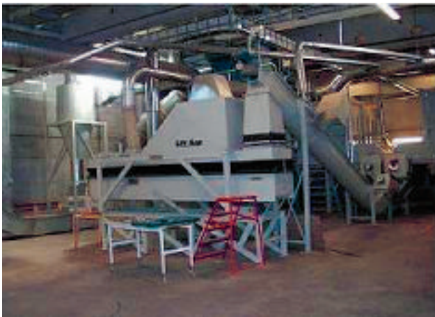
Figure 51. Left, gravimetric separator for commercial use. Right, schematic diagram of a gravimetric separator. An adjustable nozzle is placed at the end of the table and lifts relatively light fractions by an air stream, allowing heavier fractions like rocks, gravel and metal pieces pass by. Conversely, the equipment can be used to reduce amounts of very light and unwanted fractions.
