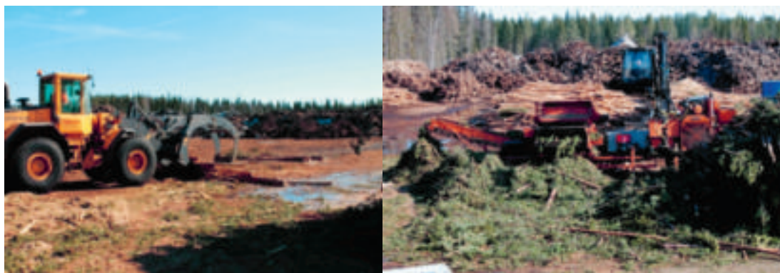
Figure 37. Left, a front-end loader and, right, a chain-flail debarking system.
