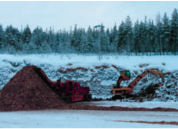
Figure 30. Stump crushing at a terminal.
