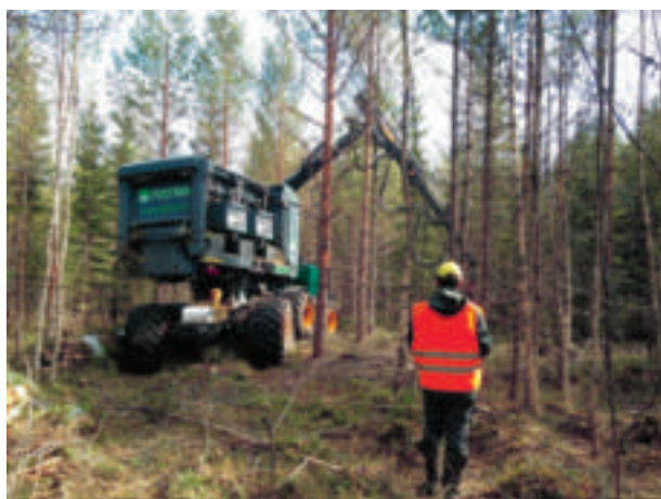
Figure 35. The Fixteri bundle-harvester system.
