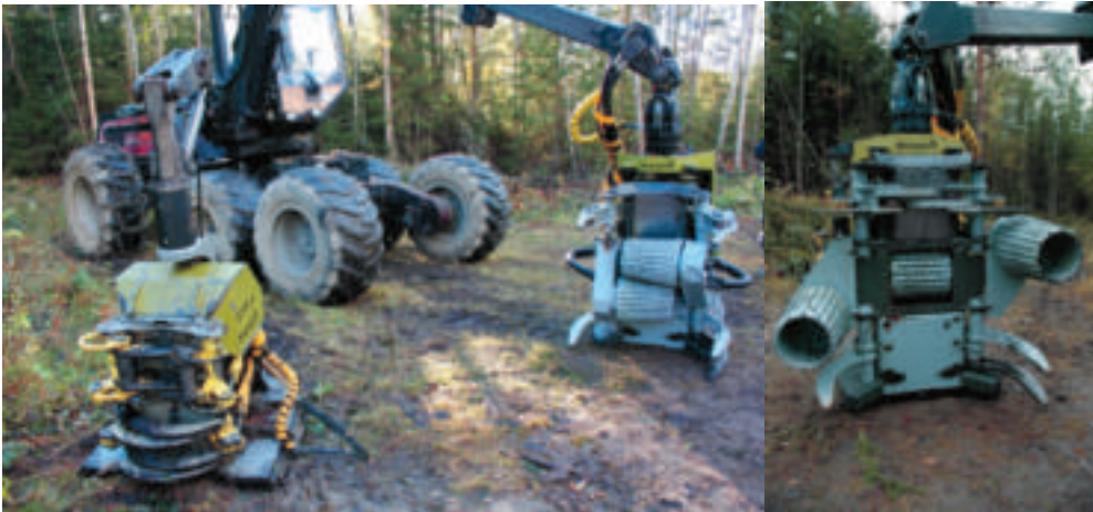
Figure 33. Left: the C16 head. Center and right: the MAMA prototype head. Both heads were developed by Bracke Forest AB, Sweden ( www.brackeforest.com ), and cut trees using a circular disc with a 3/4" saw-chain.
