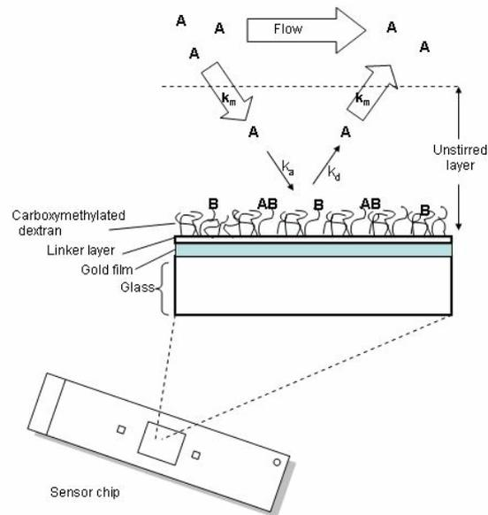
*Figure 5.* Overview of the basic interactions at the biosensor surface. The ligand (B) is attached to the surface via the flexible carboxymethylated dextran. During the association phase, analyte (A) is flowed past the surface.  $k_m$  is the mass transport coefficient used to describe the diffusion of analyte through the unstirred solvent layer.  $k_a$  and  $k_d$  are the rate constants, which describe the formation of the complex (AB).
