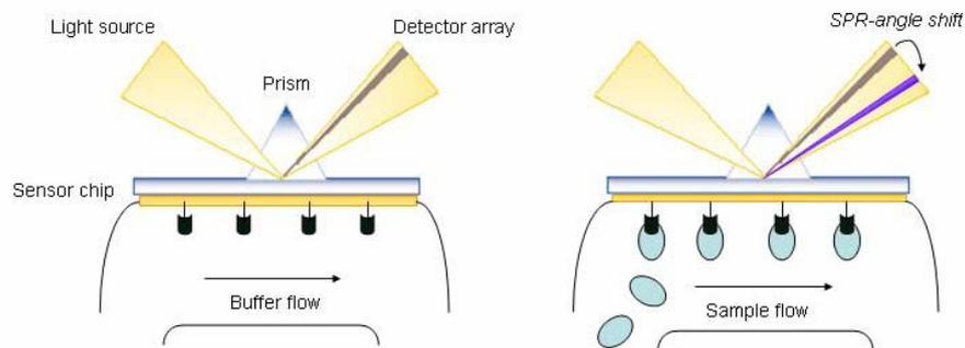
*Figure 4.* Surface plasmon resonance (SPR) biosensor principle. The binding of biomolecules to the sensor surface increase the refractive index, which induces shift of the SPR angle. The shift is directly proportional to the mass increase.
