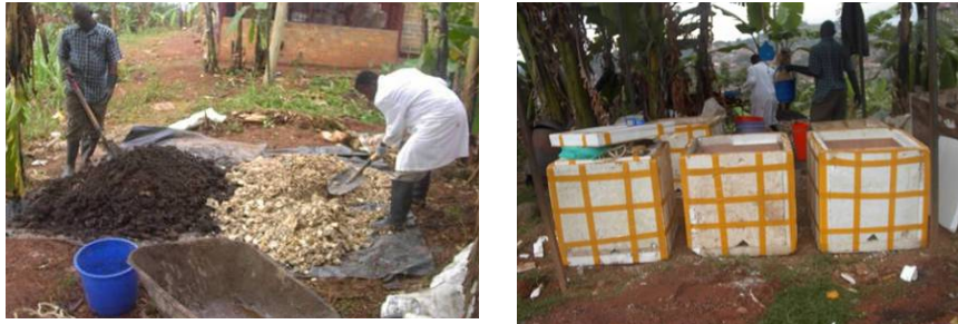
Fig. 13. Preparation of material (faeces and food wastes) for composting (left). Compost boxes used in the experiments (right) (photo: P. Kiyaga, 2006).
