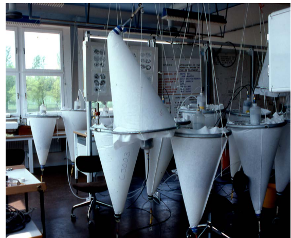
Picture 9-11. Equipment for pollen extraction of individual clones. Owing to the wind pollination of spruces and pines it is of utmost importance to take serious measures to avoid pollen contamination. Shortly before pollen dispersal, twigs are placed in the conical paper bag. When the pollen is ripe the water in the containers is emptied and the paper bag is turned upside down. Pollen drying is started by blowing dry air through the paper bag. Finally, pollen is collected in glass vessels attached at the bottom of the paper bag. Photograph Kjell Lännerholm.
