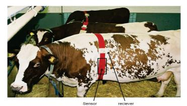
Figure: 5. Sensor and receiver used for recording the heart rate of cattle during loading for transport
